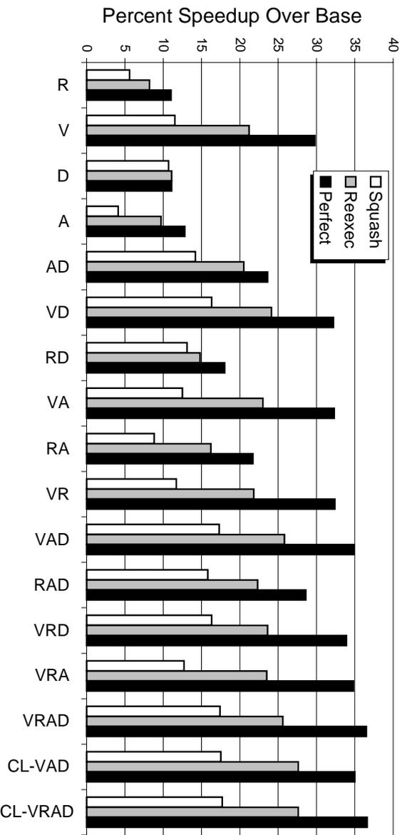
Figure 16: Average speedup results for Squash and Reexecution recovery for all combinations of the predictors using the Load-Spec-Chooser to decide which predictor to use. D = Store Set Dependence Prediction, V = Hybrid Value Prediction, A = Hybrid Address Prediction, R = Original Memory Renaming, and CL = Check-Load Prediction
