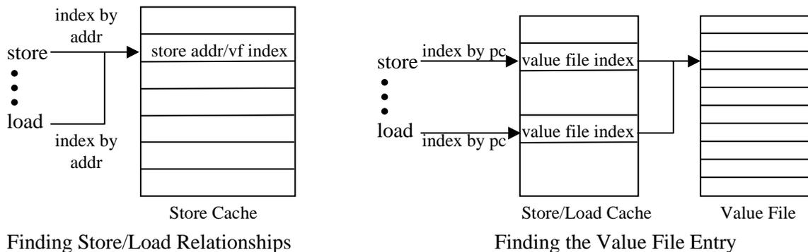
Figure 12: The structure of the memory renaming architecture [30]. The Store Cache is used to find the relationships between store and load instructions. The Store/Load cache is used to keep track of which Value File entries to use for store and load instructions. Store instructions use the value file entry to store their last value or a pointer to the instruction producing the value. Load instructions used the value file entry to predict the value to use for the load.
