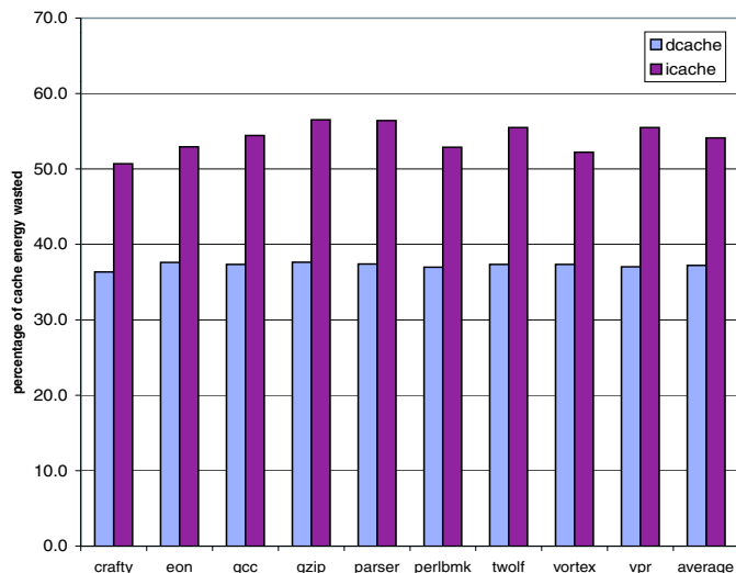
Figure 5: Potential cache energy savings with optimal cache sizing for the integer benchmarks.
